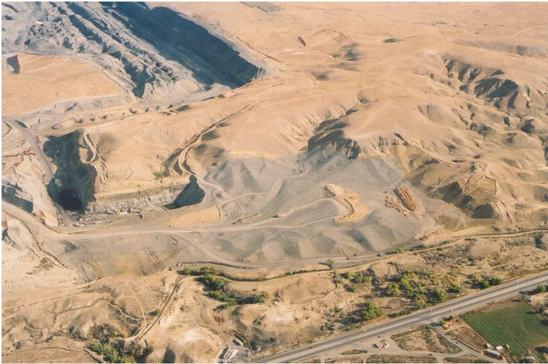
Figure 7. Fluvial geomorphic reclamation is underway at the 115-acre Cottonwood Reclamation Project, Farmington, New Mexico. Gray colored material is mine spoil being graded using fluvial geomorphic approach. The U.S. Department of the Interior awarded San Juan Coal Company "National" and "Best of the Best" reclamation awards for 2004 for this project.
