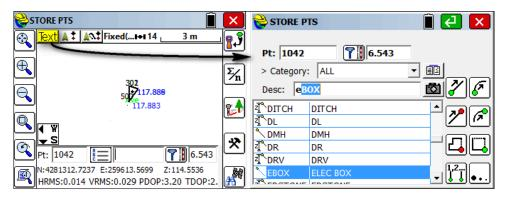
The Text screen uses a large character size for easy viewing, and limits options to Monitor/Skyplot, Configuration, Offset, and Store. You can return to the graph view by tapping the GRAPH button. You can also temporarily view your points on the screen by tapping Map, then tap Back to return to the text-based data collection screen. Note that the program will remember which screen you were in last (Graph or Text) and return to that mode of data collection automatically.
